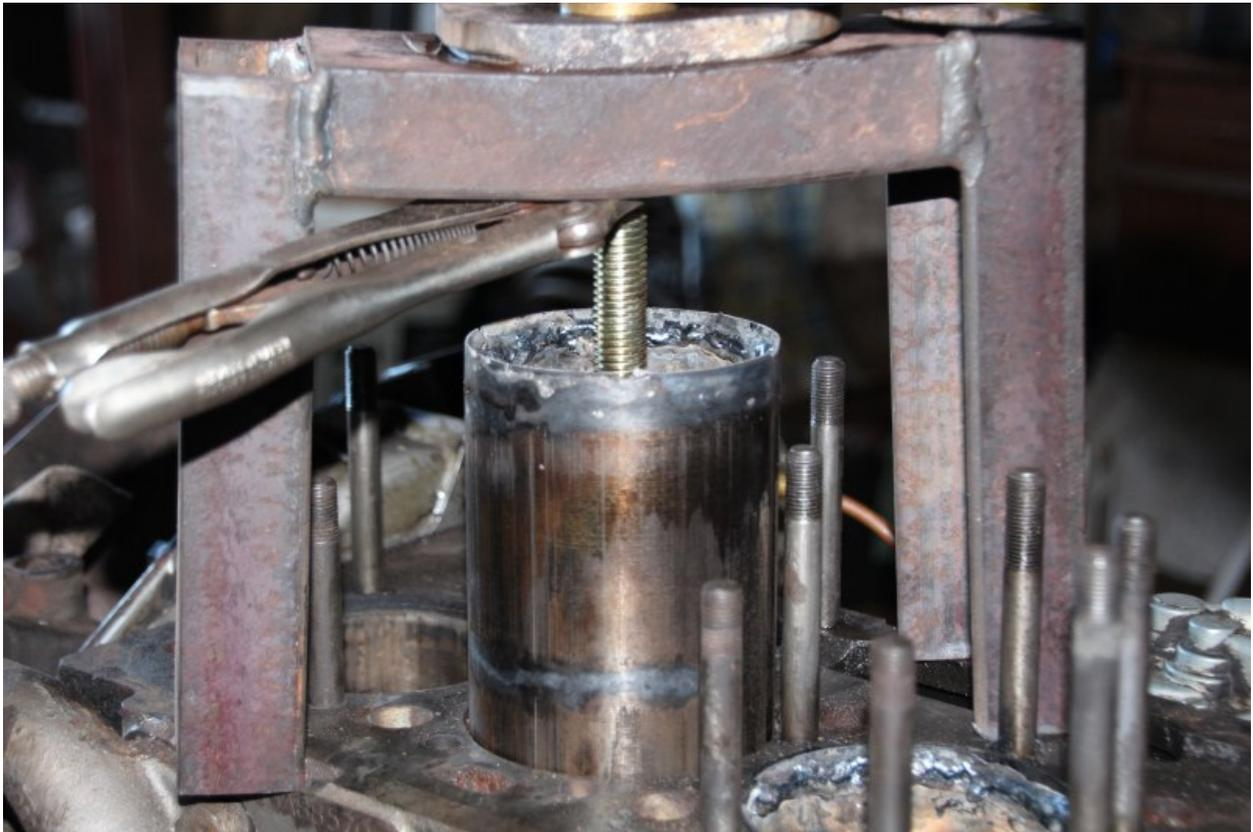
Here the liner is about half way out - watch for the vice grips and or liner top to contact the puller frame.
