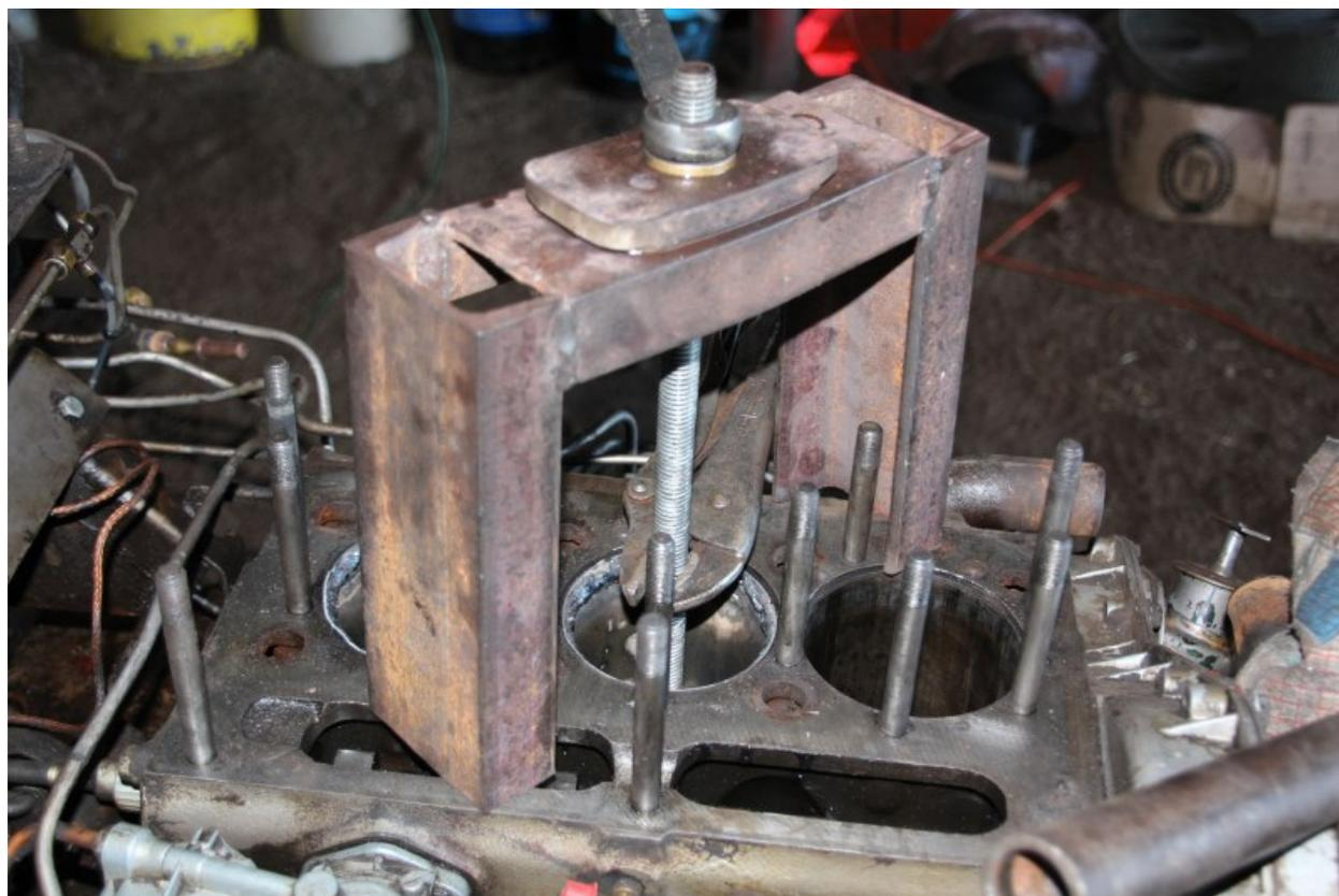
Even after the welding the liners can be very hard to pull. A minimum of 5/8 reddi rod should be used with a well built pulling frame. It must be positioned on the block carefully so the pulling point is centered and so that it won't slip off. It may be necessary, after putting pressure on the puller, to tap the bottom of the puller with a hammer and long punch from underneath ( careful - don't hit the crank shaft in doing this inframe ).
