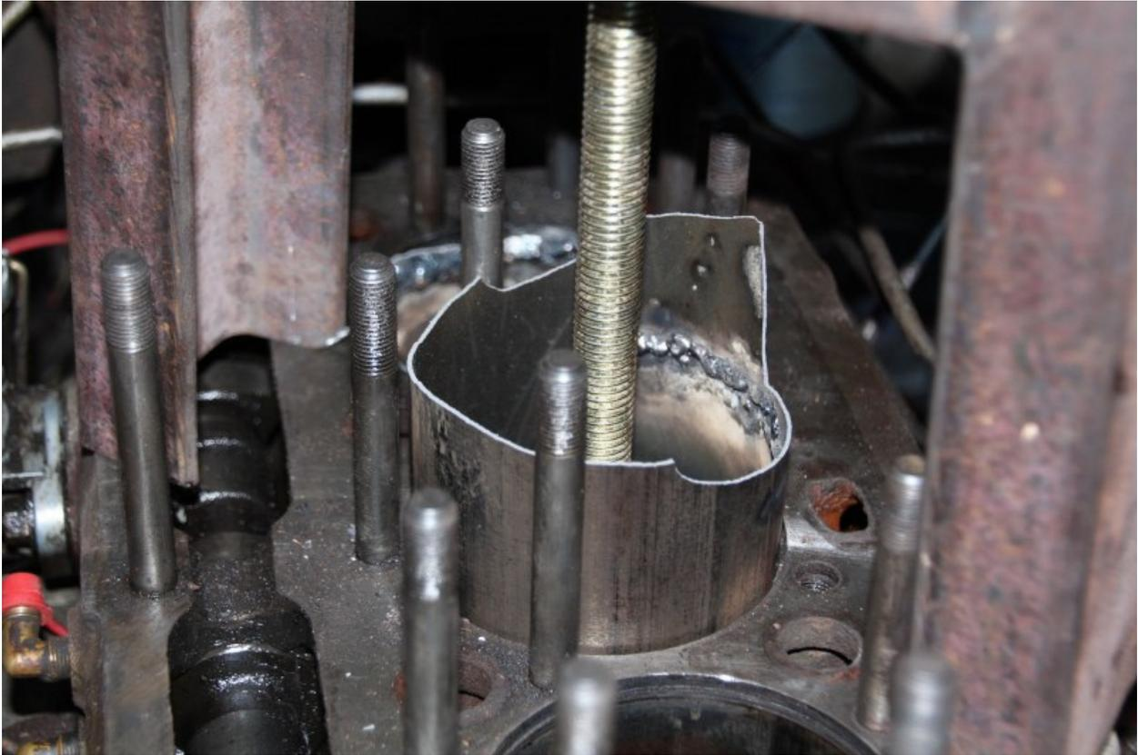
When the liner contacts the puller frame it should be broken off (they break very easily with a tap of a hammer ) so that you can continue pulling. A tall pulling frame could be used but the taller it is the stronger it has to be and the longer the reddi rod. I found that a shorter puller and two pulling stages works best.
