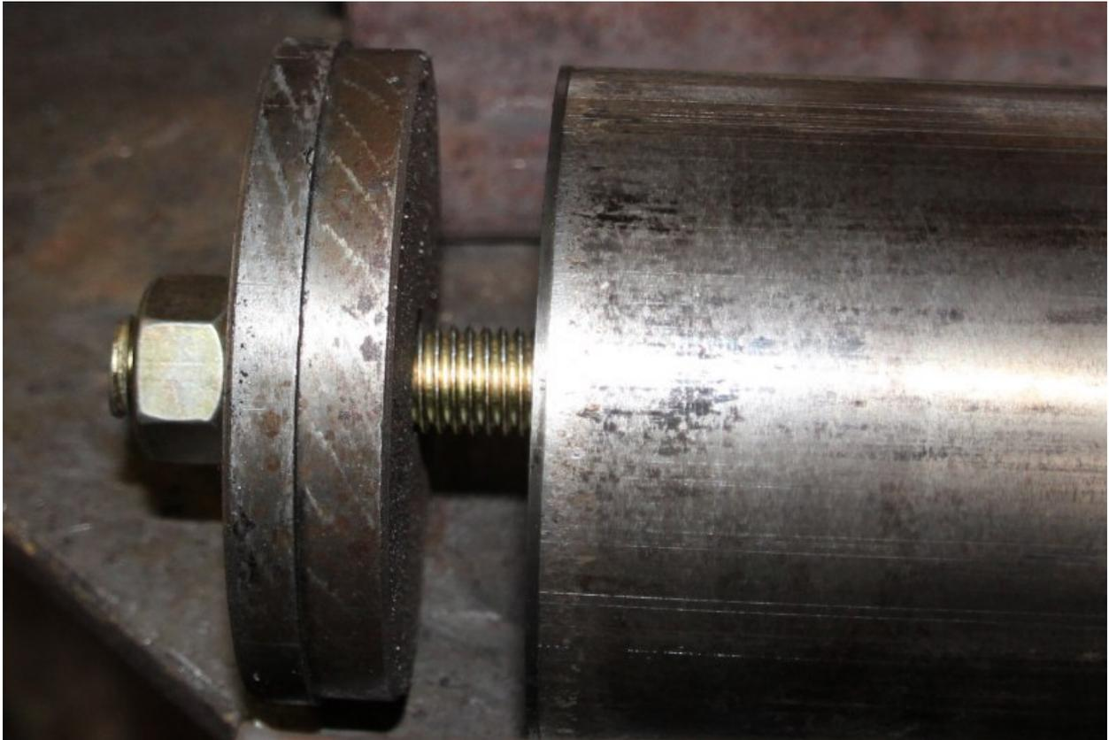
The puller must use an exact sized bottom plate. It must be stepped so that the top of the plate fits inside the liner with no play. The lower section must be slightly smaller than the OD of the liner. The step must be machined precisely to give an even pull.
