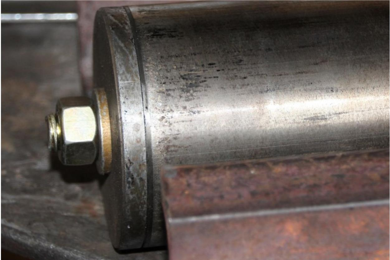
The bottom plate must be fitted squarely into the liner bottom before pressure is applied.
