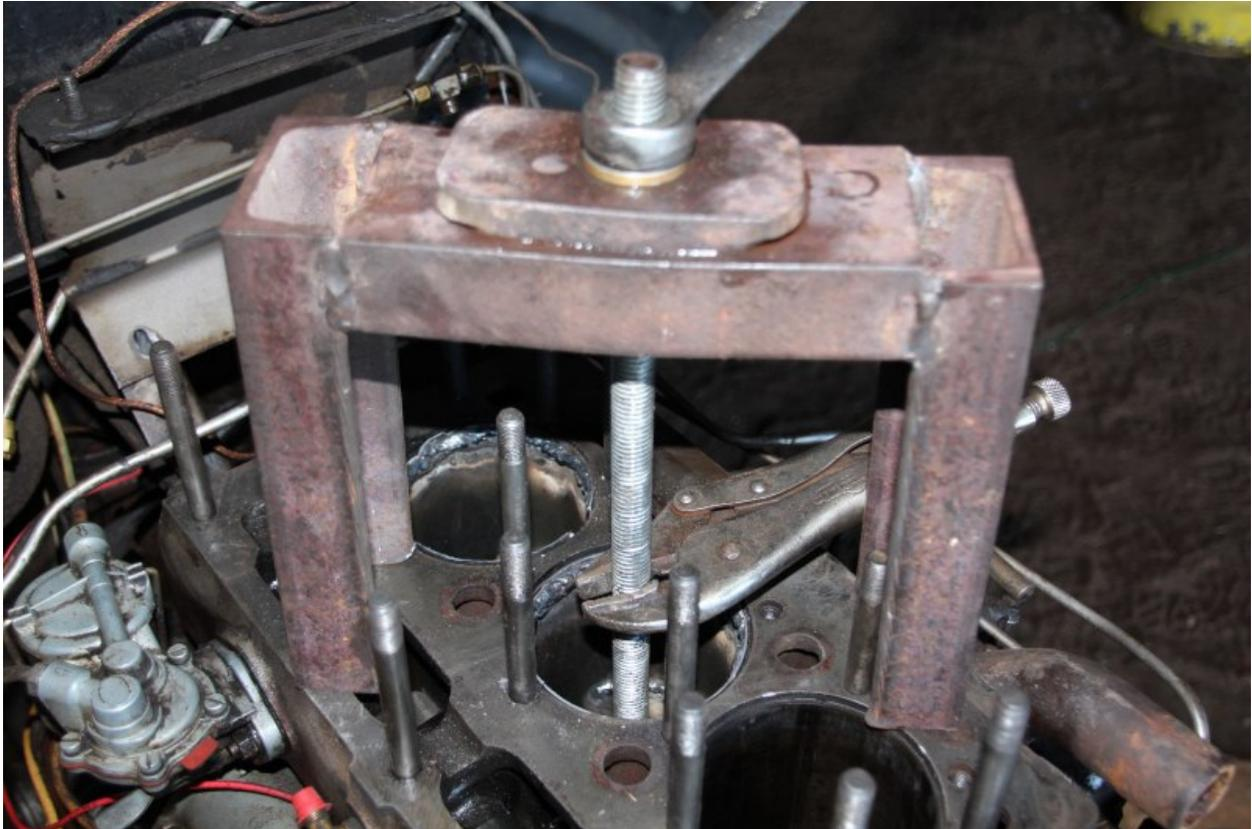
Vice grips should be placed on the reddi rod to stop it from turning. It could spin and not pull or it could spin and screw down into the crank shaft ( if doing the rebuild in frame ).
