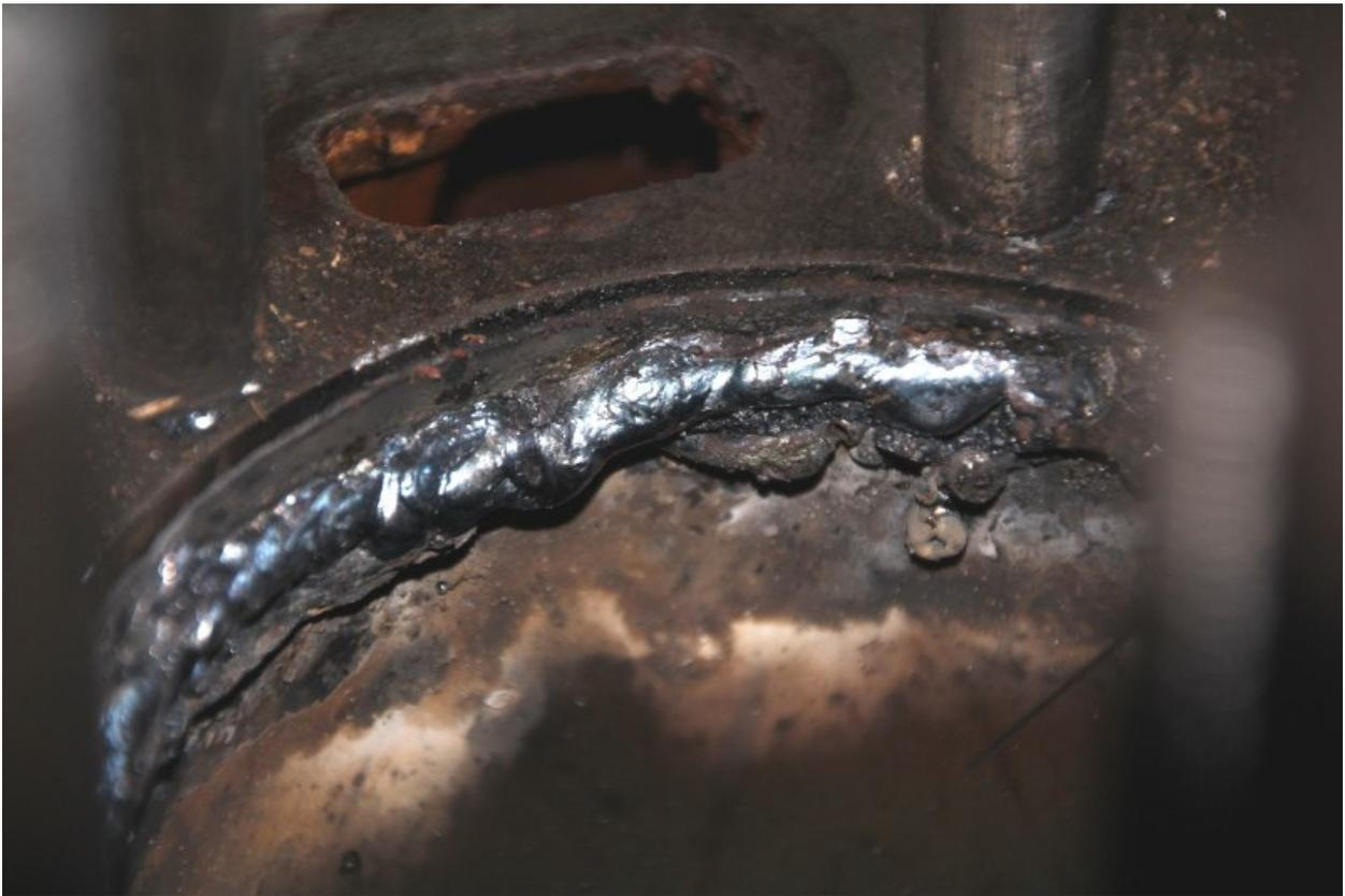
Welding a bead around the inside of the liner can shrink the liner to make it easier to pull. Extreme caution must be used however as the liner are very thin and you must not burn through.
